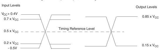
Figure 10.1 Input, Output, and Timing Reference Levels
